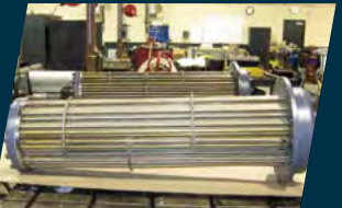
Heat Exchanger Retubing & Repair
